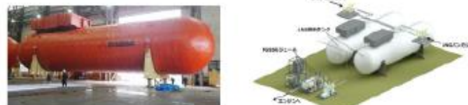
Current LNG fuel tank and fuel supply system
