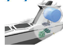
Image of hydrogen fuel tank and fuel supply system
