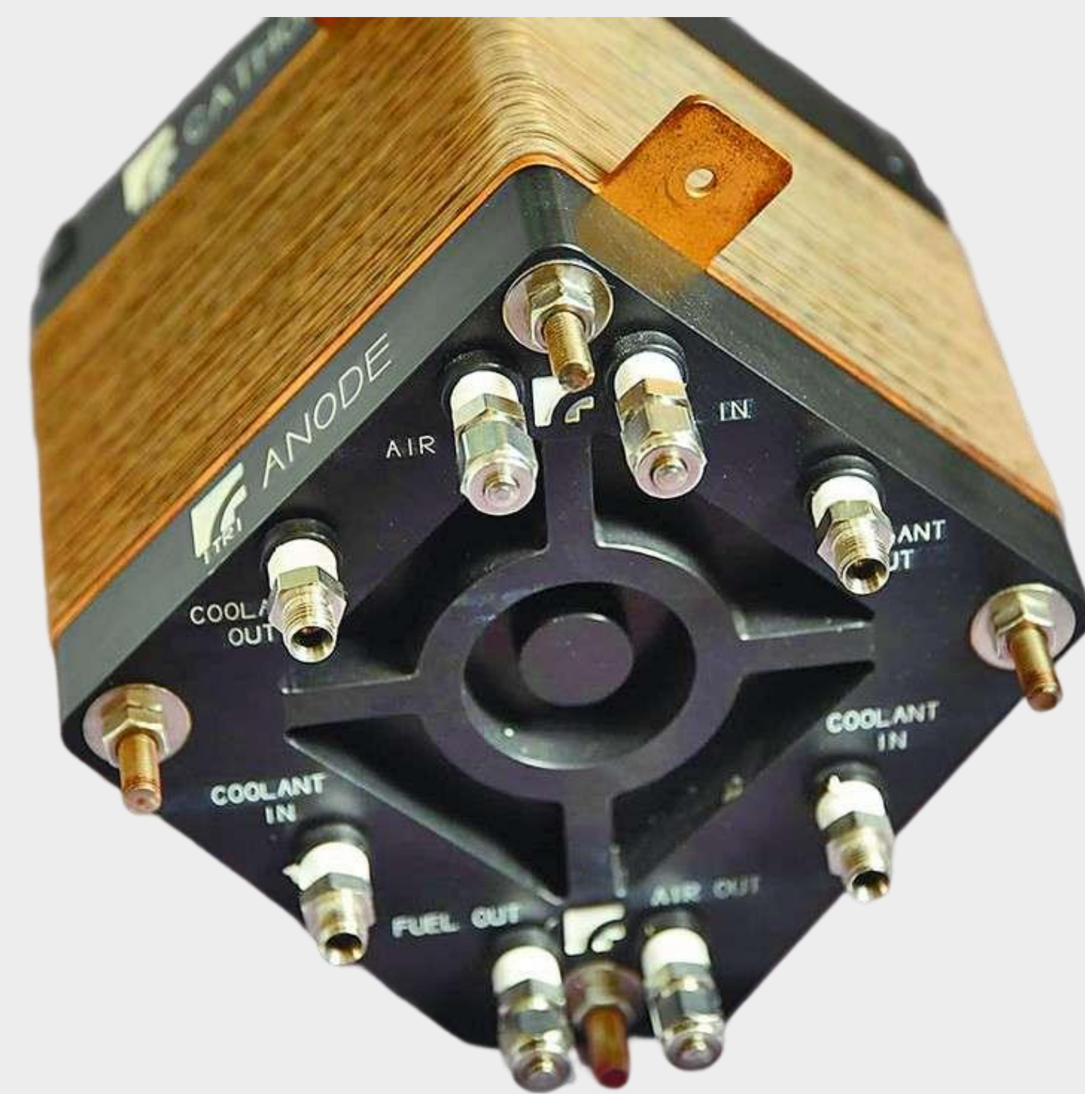
Light weight fuel cell with metal bipolar plate
