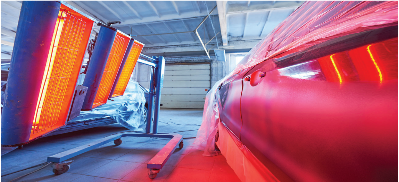
Figure 2C-1. An infrared dryer for automobile paint. Short-wave infrared emitters can reach filament temperatures of 2,000°C. (Dmitry Kalinovskiy/Shutterstock.com)
