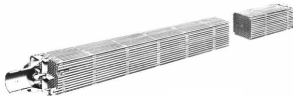
Figure 10-2. Boiling water reactor fuel bundle. 9
